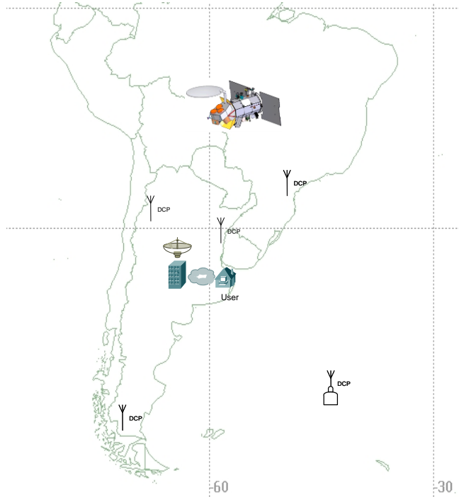
DCS main components Source CONAE
