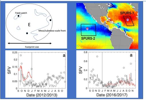
Upper left: Schematic showing a satellite footprint, some characteristic SSS variability, the estimation point for the satellite ("E") and three in situ validation measurements.
