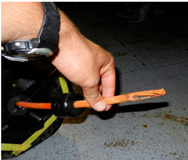
Figure 6.5: The damage to the wire rope jacketing indicates that corrosion was the leading cause for the mooring to fail.
