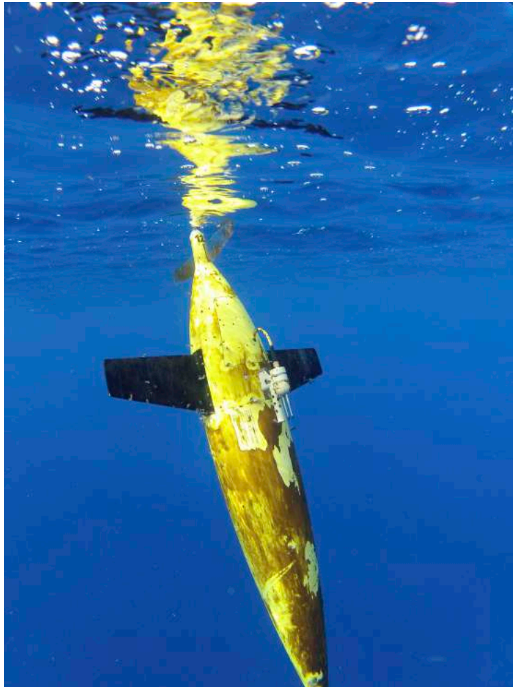
Figure 8.1: Seaglider 122 just prior to recovery.
