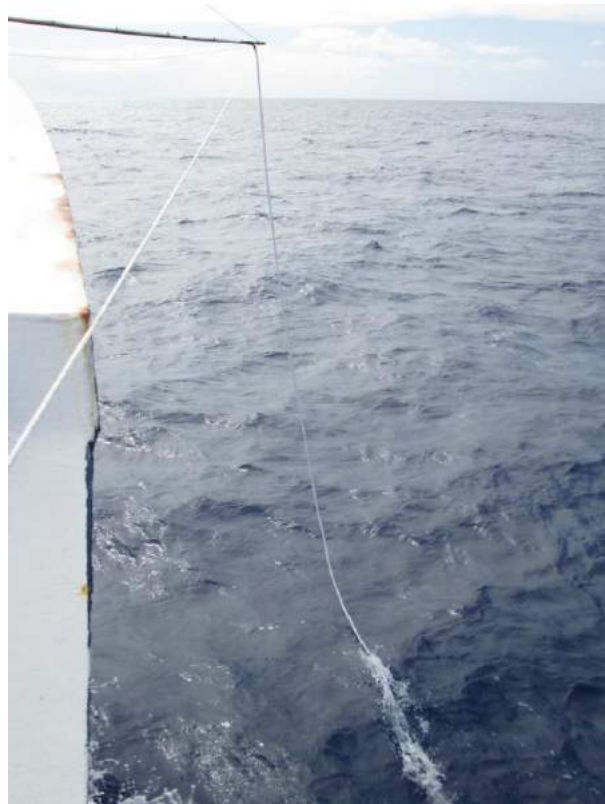
Figure 4: The SST snake mounted on the windsurfer mast at the starboard bow. The halyards were fastened forward, at the met mast forestay, aloft, at the met mast and aft, at the railing (visible as white line in this image). Picture used with permission by Alec Bogdanoff.
