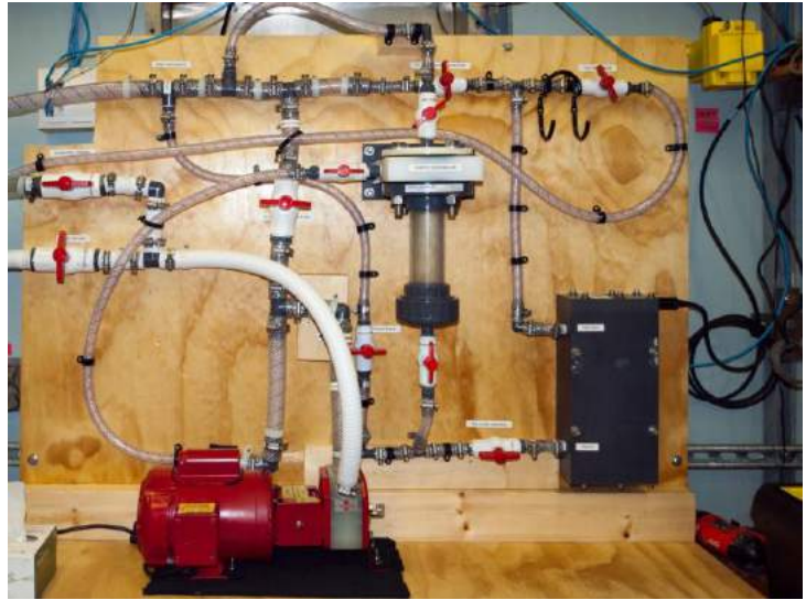
Figure 3: The salinity snake shipside system after modifications to include a cursory de-bubbling in the pump discharge. Note that in this picture, the system is set to use ship-supplied seawater for cross-calibration.
