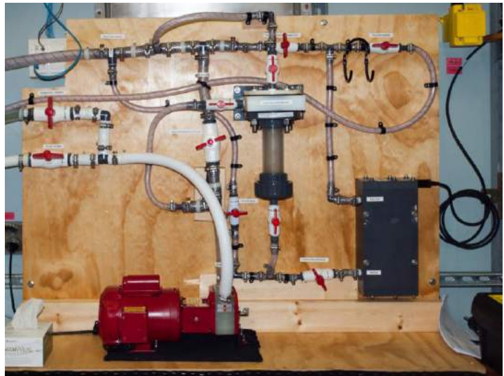
Figure 2: The vessel-side of the sea surface salinity snake, consisting of intake control (right), pump (bottom), de-bubbler (middle) and SBE-45 TSG (left) as well as discharge, priming and bypass controls.
