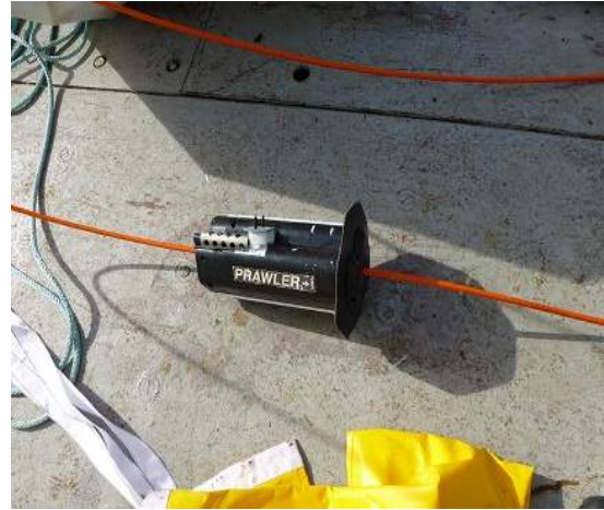
Figure 2.a. (left) Surface float for Prawler mooring. Figure 2.b. (right) Prawler unit on jacketed cable. It contains the CTD, inductive modem and ratchetting mechanism.
