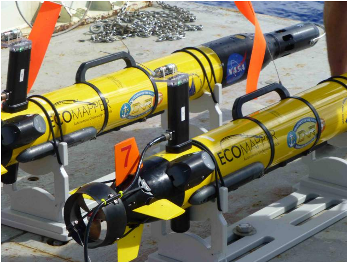
Figure: Ecomappers on deck, just prior to deployment from the fantail of R/V Knorr.
