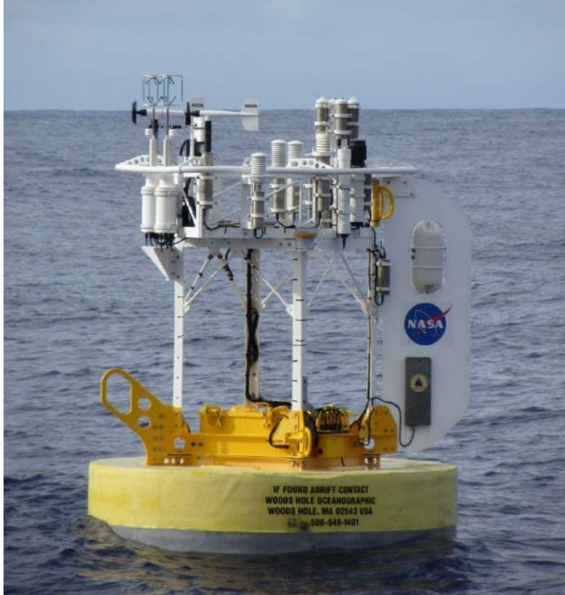
Figure X2: WHOI-SPURS surface mooring after deployment.
